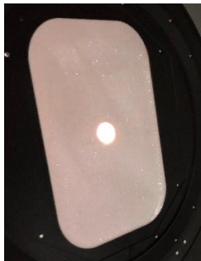
Measured shading fabric sample in photogoniometer sample holder
