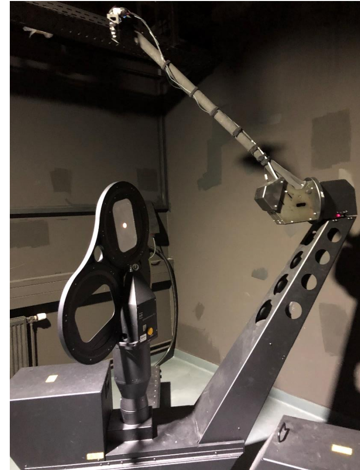
pgII photogoniometer with measured shading fabric
