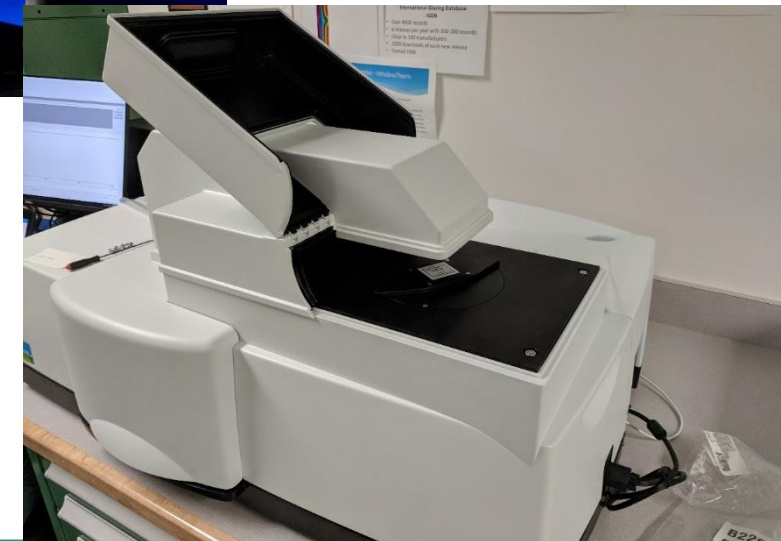
Commercial spectrophotometer with new integrating sphere at LBNL
