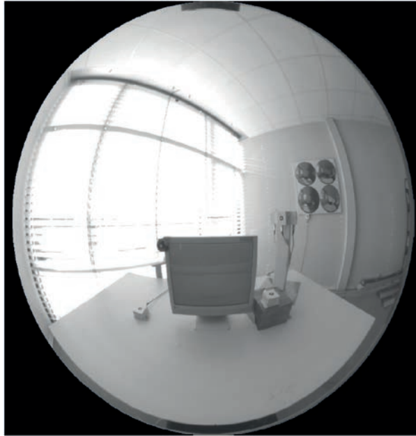
FIGURE 17 - Example of glare caused by a high luminance level of the window
